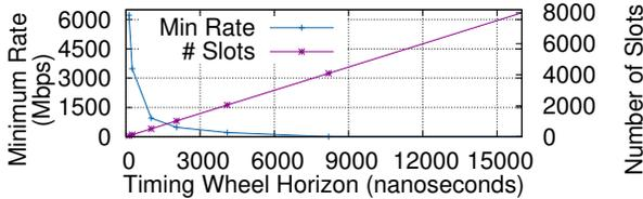
Figure 17: An analytical behavior of the minimum supported rate for a specific Timing Wheel horizon along with the required number of slots for a slot size of two microseconds.
