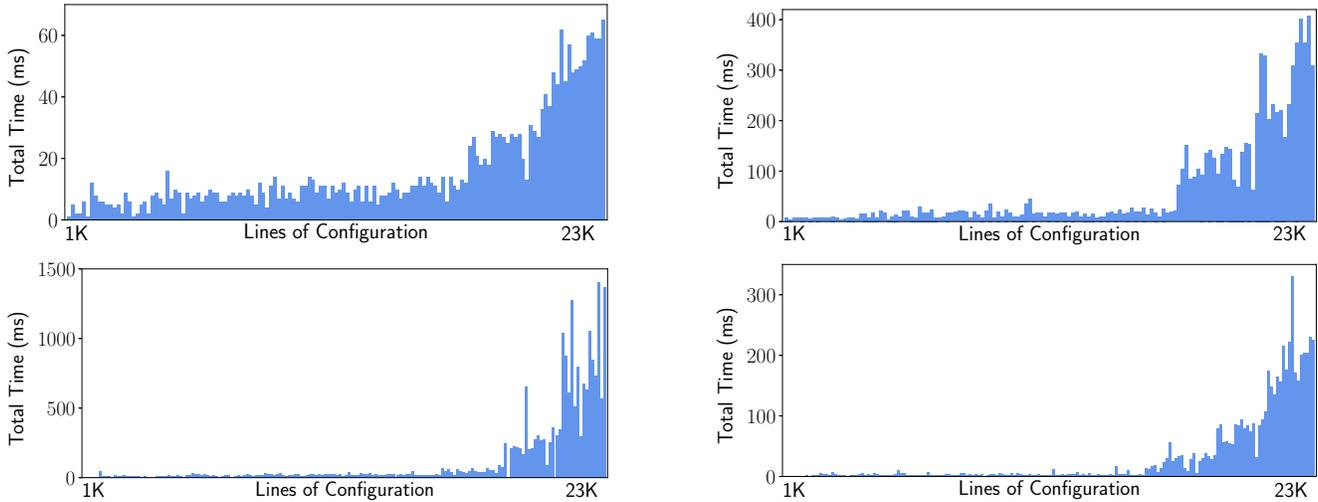
**Figure 7: Verification time for management interface reachability (upper left), local equivalence (upper right), blackholes (lower left), and fault-invariance (lower right) for real configurations sorted by total lines of configuration.**
