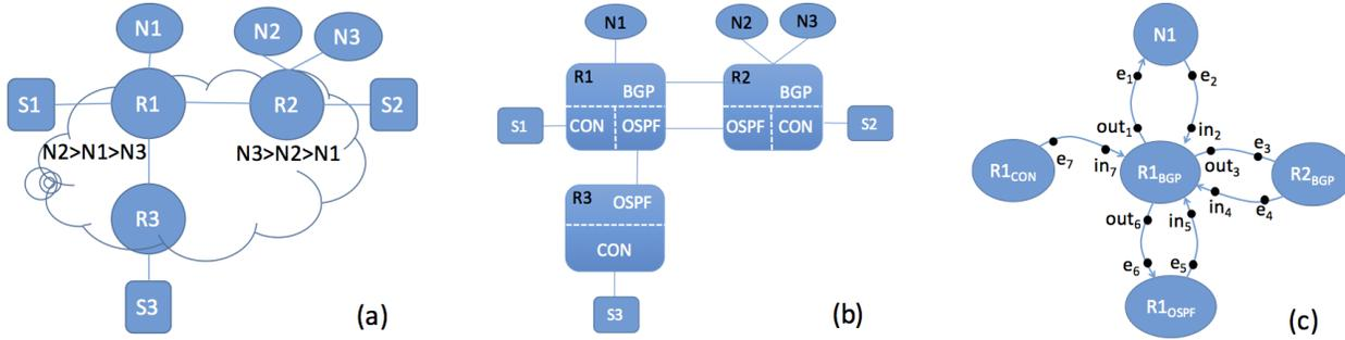
Figure 2: (a) An example network. (b) Its protocol-level decomposition. (c) Routing information flow for BGP at R1.
