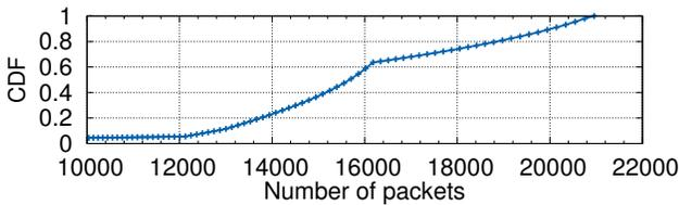
Figure 8: Buffered packets of a VM at a shaper in hypervisor. The bump in the curve is because there are two internal limits on the number of buffered packets: 16K is a local per-VM limit, and 21K is at the global level for all VMs. There are packet drops when the 16K limit is exceeded, which impacts the slope of the curve.
