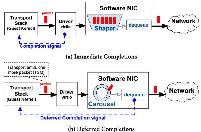
**Figure 11: Illustration of Completion signaling.** In (a), a large backlog can build up to substantially overwhelm the buffer, leading to drops and head-of-line blocking. In (b), only two packets are allowed in the shaper and once a packet is released another is added. Indexing packets based on time allows for interleaving packets.
