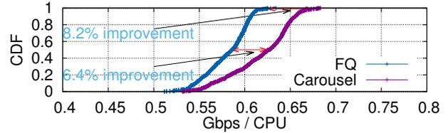
Figure 21: Comparison between FQ and Carousel for two machines serving large volumes of video traffic exhibiting similar CPU loads showing that Carousel can push more traffic for the same CPU utilization.
