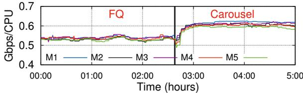
Figure 20: Immediate improvement in CPU efficiency after switching to Carousel in all five machines in a US west coast site.
