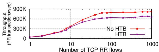
Figure 6: TCP-RR rate with and HTB. HTB is 30% lower due to locking overhead.
